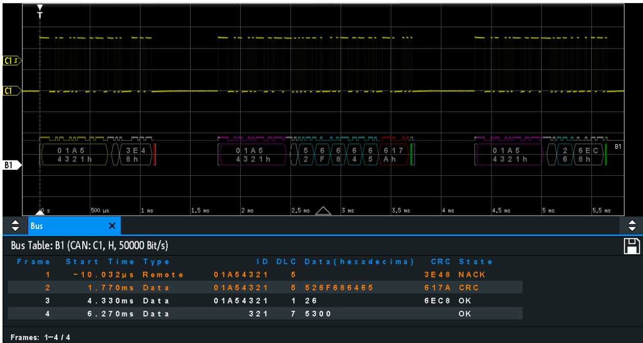
Figure 13-24: Decoded CAN signal with bus table, trigger on frame start
